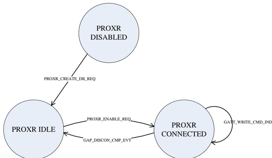
From the above figure Proximity Reporter task has three states. The arrows show the messages that will be processed in each state. The following snippet is created based on state machine.
