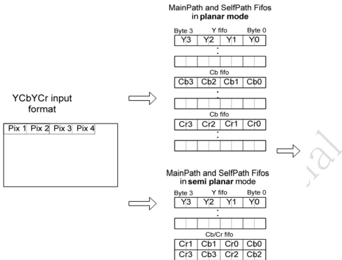
Fig. 31-5 Storage Scheme in Planar and Semi-planar Mode
