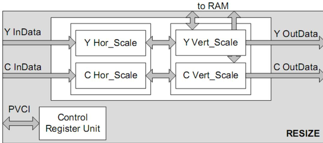
Fig. 31-2 Block Diagram of the Resize Module
