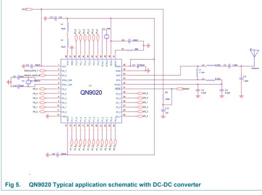
For application using battery supply, it is highly recommended to apply the circuit for QN9020 with internal DC-DC converter.
